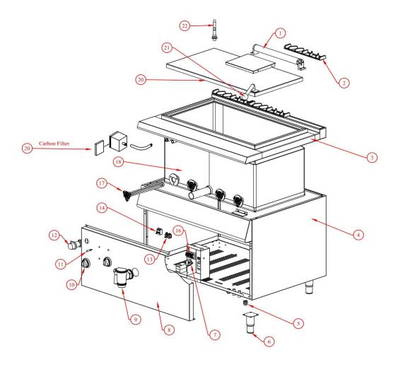
Note: Please change the carbon filter every 6 months to prevent oil odor. The filter is under the front panel.
